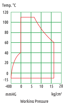
F83DJ16 DN350 ... DN600 Burst Pressure 48bar
