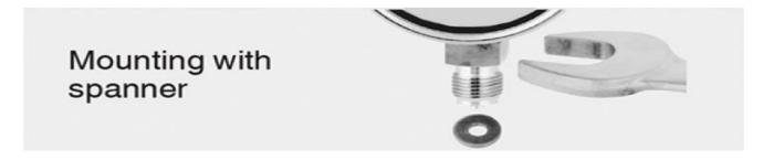
Correct sealing of pressure gauge connections with parallel threads ① must be made using suitable sealing rings, sealing washers or profile seals. The sealing of tapered threads (e.g. NPT threads) is made by providing the thread ② with additional sealing material such as, for example, PTFE tape (EN 837-2).
