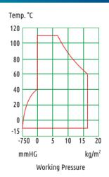
F85DJ-I DN15 ... DN50 Burst Pressure 48bar
