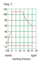
F85DJ-I DN15 ... DN50 Burst Pressure 60bar
